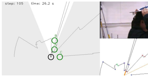
(b) Case of occlusion, as seen by the robot. Target A is passing in front of target B while the robot R is turning.
