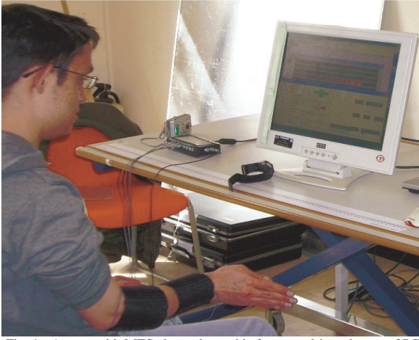
Fig. 1 - A user, with MES electrodes on his forearm, drives the car of PC game using hand gestures
