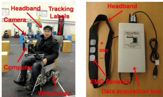
Fig. 2 Intelligent wheelchair setup for subject and indoor experiment environment (Left) and the Cyberlink TM headband and data acquisition device (Right).
